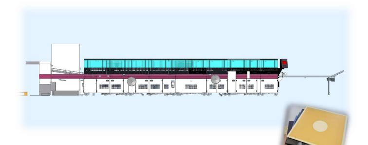
W+D 802.04 Record-Sleeve machine for the production of Vinyl Record Jackets, Gate-fold covers and Inner sleeves with center hole
